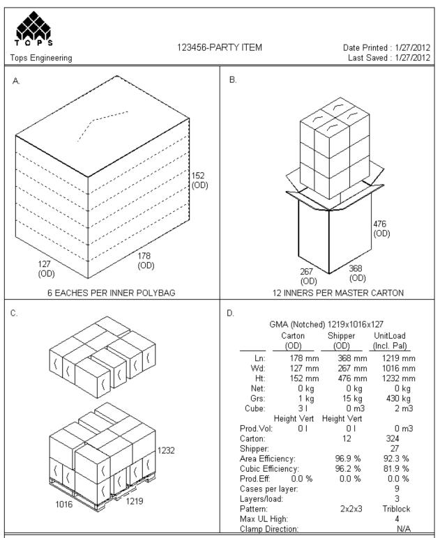
Notes: Inner is a 3 mil polyethylene bag. Close and securely tape the polybag to prevent the eaches from falling out. Master carton must be able to pass a 200 lbs/in2 bursting test or a 48 lbs per inch edge crush test. All
